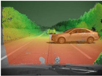
6 Depths-reconstruction from binocular stereo (Figure: Daimler AG)
