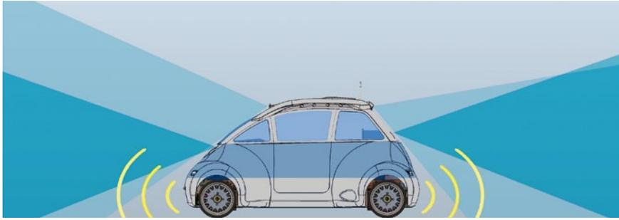
2 Rear and front camera coverage and ultrasound
