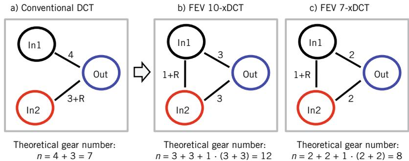
① Five steps (red) of systematic gear set synthesis (upper part) but also gear set structures a, b and c of conventional DCT, FEV 10-xDCT and FEV 7-xDCT (lower part)
