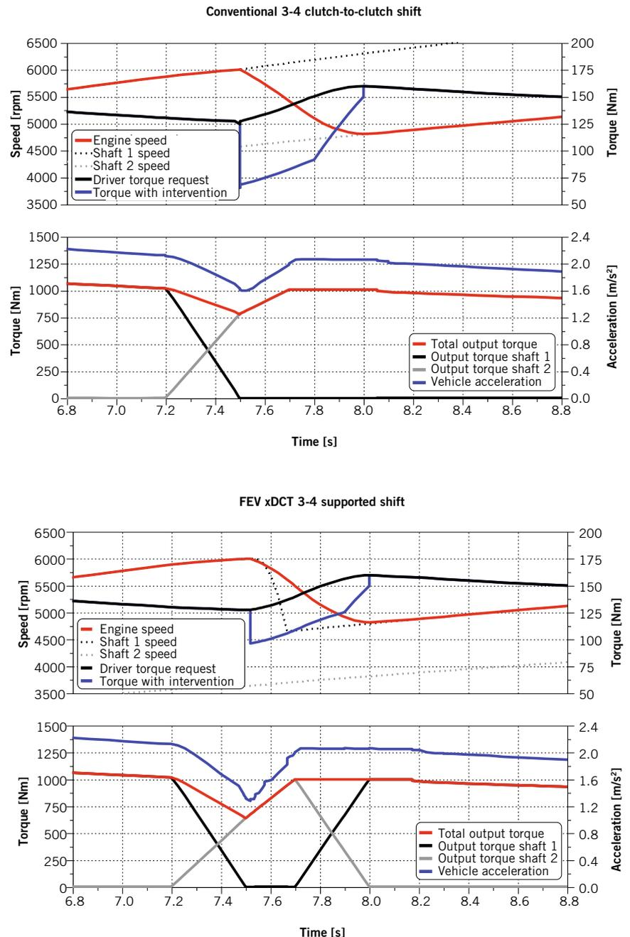
③ Comparison of the conventional DCT shift to the supported shift of the FEV 7-xDCT (3<sup>rd</sup> gear → 4<sup>th</sup> gear)
