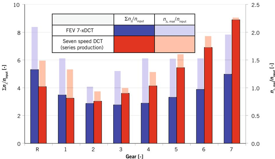
5 Delta speeds at non-engaged idler gears for the FEV 7-xDCT and a series-production seven-speed DCT
