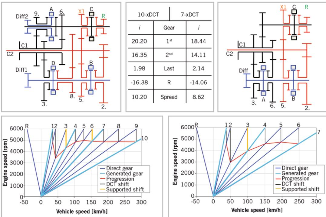
② Gear set layouts and exemplary ratio stepplings of 10-xDCT (left) and 7-xDCT (right)
