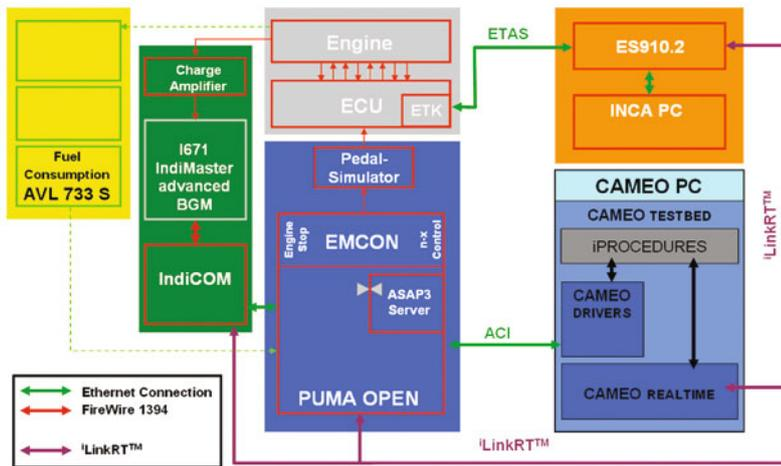
Figure 6: Future test bed set up with iLinkRT
