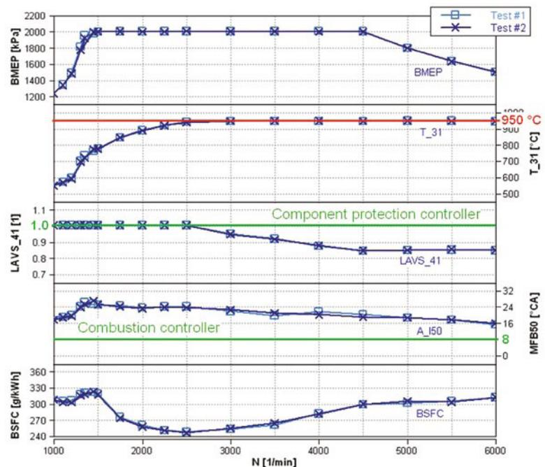
Figure 3: two repetitions of full load measurements on one supercharged gasoline engine using real time controllers
