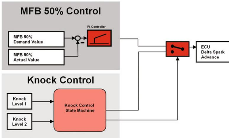
Figure 2: Real time control example: Combustion controller
