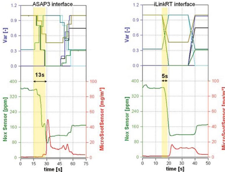
Figure 5: ECU parameter ramps with ASAP3 in comparison with iLinkRT interface
