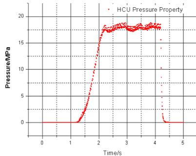
**Fig. 4.** The pressure property of ESC HCU
