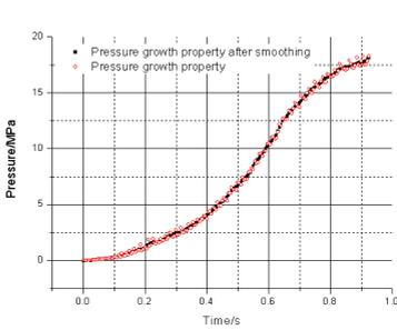
Fig. 5. The pressure increase property ESC HCU
