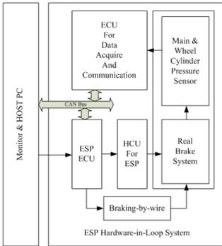
Fig. 1. The scheme for ESC HiL
