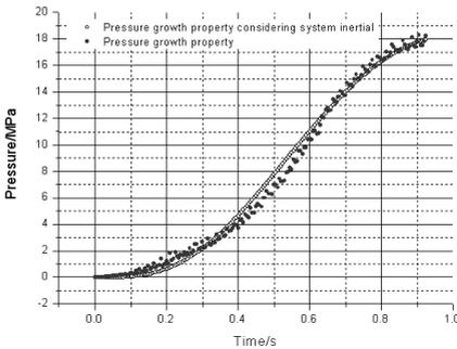
**Fig. 7.** The pressure increase property after parameter identifying
