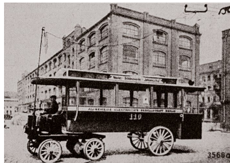
FIGURE 3 AEG experimental car with overhead line from 1898 (© Springer Vieweg)
