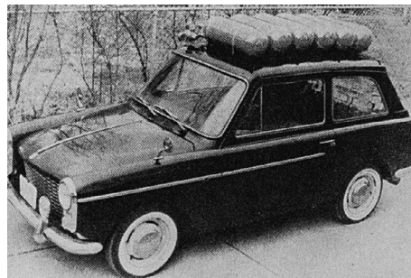
FIGURE 4 The Austin A 40 as a test vehicle with fuel cell drive from 1971 (© Springer Vieweg)
