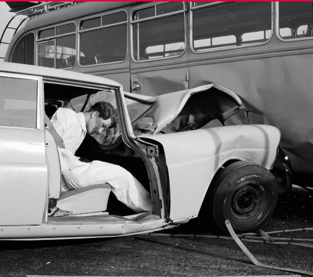
1959 Crash tests in the Mercedes plant in Sindelfingen (Germany) with cars from the W111 model range (1959 to 1965). The so-called Fintail is the first car in the world with a rigid passenger compartment (© Daimler)
