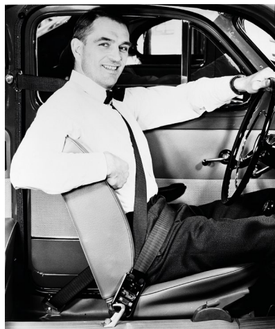
FIGURE 2 The hunchback Volvo in 1959 was the first production model to be fitted with a three-point seatbelt (© Volvo)
