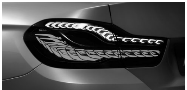
2015 The BMW Concept M4 Iconic Lights model with the first OLED rear lights (© BMW)
