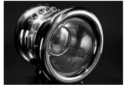
1908 Acetylene gas headlight with a parabolic reflector and a lens with a reflective coating (© Hella)
