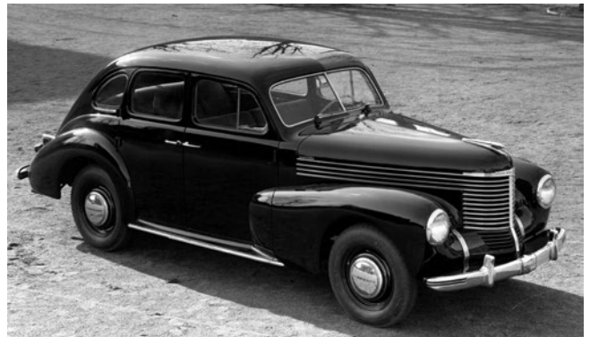
1948 Although curved windshields were invented in Germany in 1921, split screens, like this one in the Opel Kapitän, remained in use for many years (© Opel)
