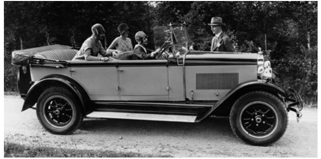
1928 Wanderer W 11 touring car: A tiltable windshield and hinged glass draft deflectors at the sides tell tales of drives at a leisurely pace (© Audi)
