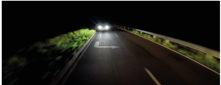
FIGURE 2 Turn-by-turn directions from the navigation system can be displayed in good time (© Ford)
