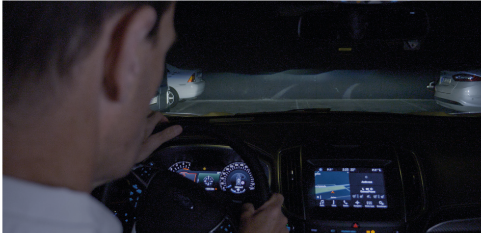
FIGURE 4 The display of lane markings could make it easier to keep in lane (© Ford)
